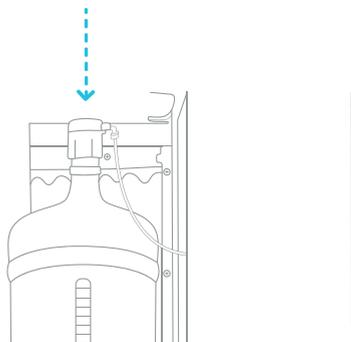
7. Slide the collar down until it clicks into place. If you are using a 3 gallon bottle rather than a 5 gallon bottle you can adjust probe by pressing the two tabs at the head of the probe and sliding the collar down to the neck of the bottle.
