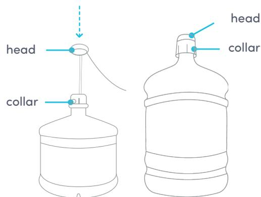
8. Push the head down until the tube hits bottom of the bottle.
