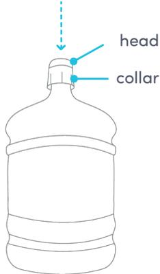
7. If you are using a 3 gallon bottle rather than a 5 gallon bottle you can adjust probe by pressing the two tabs at the head of the probe and sliding the collar down to the neck of the bottle.
